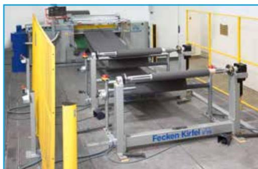
Splitting Machine K 21 and R 10 and two R 39.
