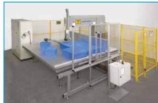
Vertical Bandknife Cutting Machine V 51/5.
