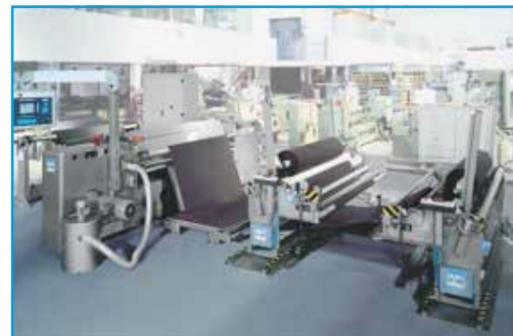
Splitting Machine G 11 with wind-up and wind-off device.
